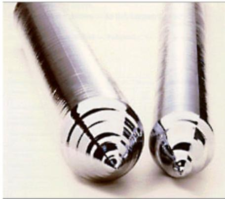
**Figure 4.** Deux lingots de silicium monocristallin [8]
