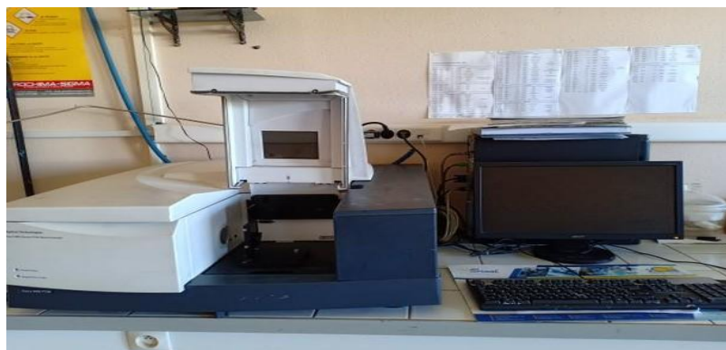
Figure 8: l'appareil FTIR Agilent Technologies Cary 600.
