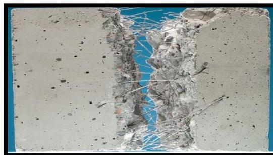
Figure 20: Béton fibré<sup>33</sup>
