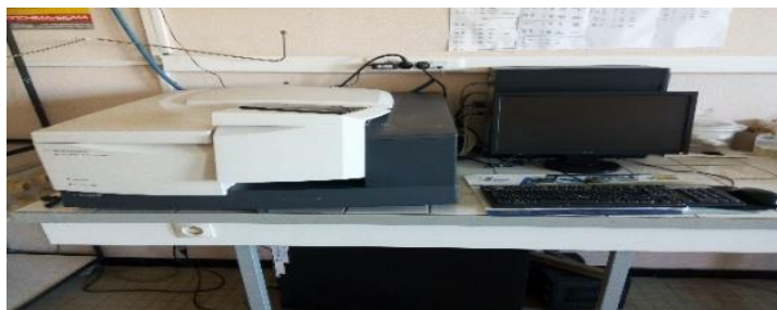
Figure II.6. Agilant technologies Cary 640 série IRTF
