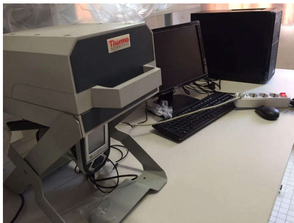
Figure II.8 : Appareil XRF de type Thermo scientific Niton XL3t
