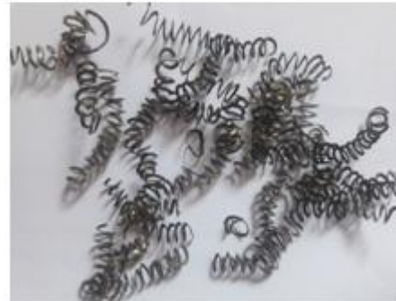
(o) : V_c = 130\text{m/min} p = 2\text{mm} a = 0.64\text{mm/tr}
