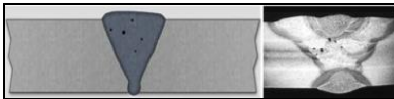
Figure III.20 : Inclusions gazeuses porosités uniformes
