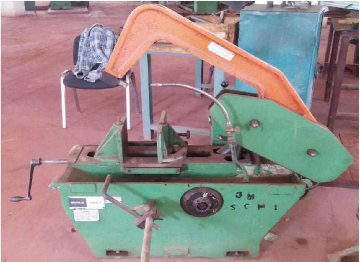
**Figure I.11** Scies alternatives horizontales ALMO SMA3
