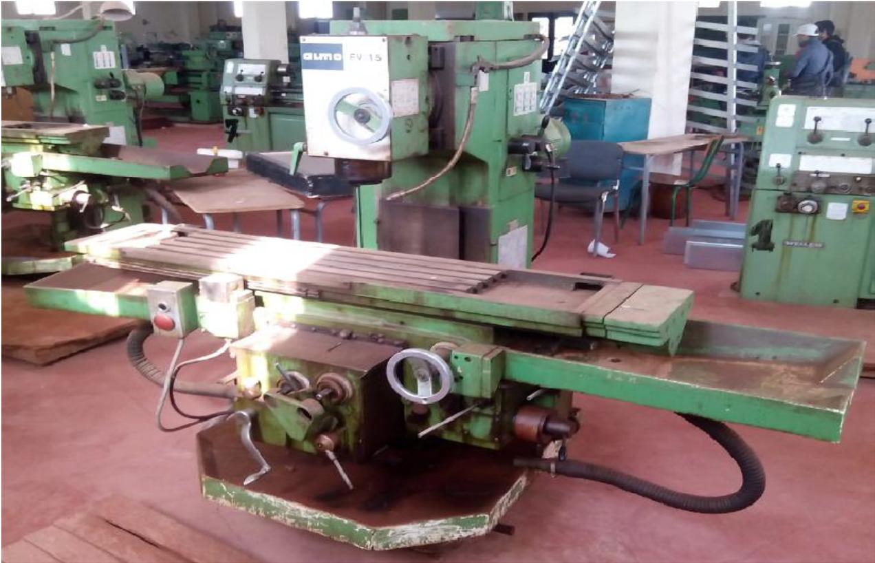
**Figure I.7** fraiseuse verticale PMO FV 2.5
