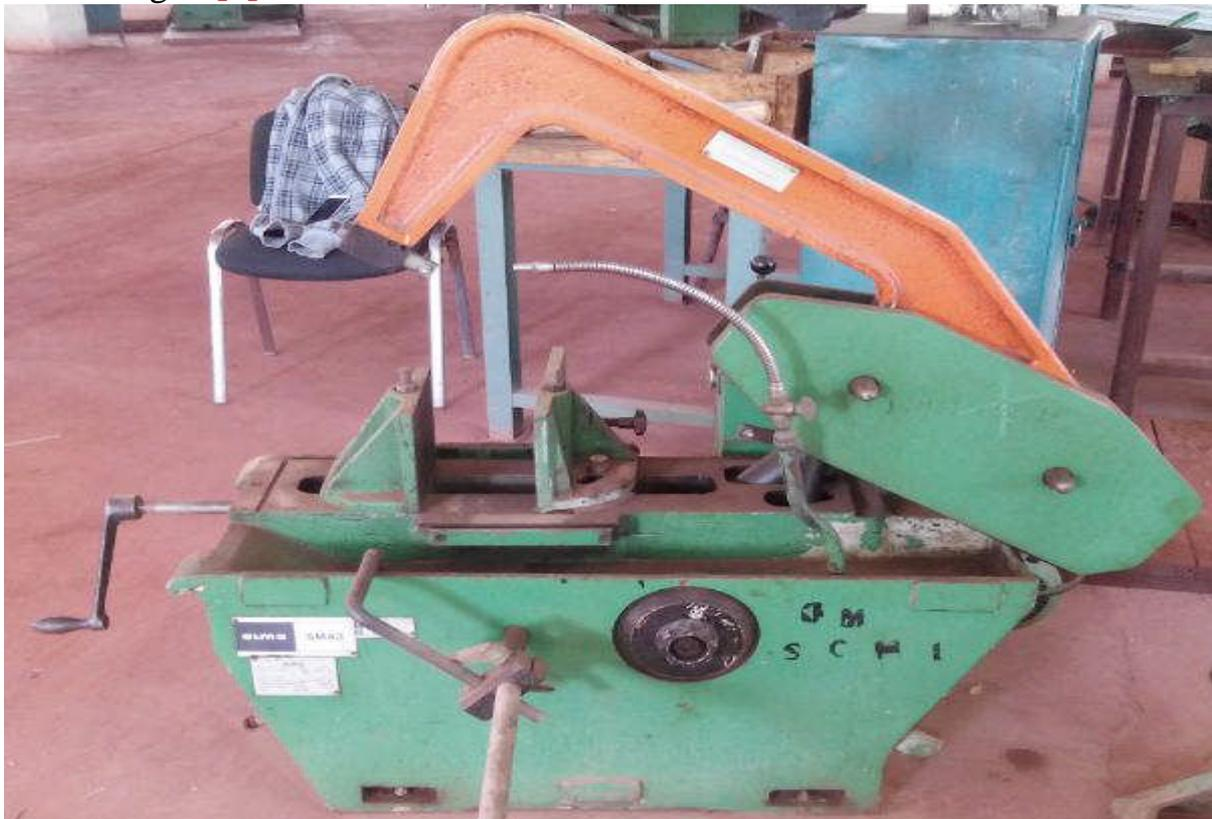
**Figure I.10** scie alternative horizontale ALMO SMA3
