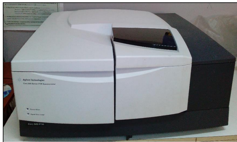
Figure II.3 : Appareillage FTIR utilisé (AGILENT technologies).
