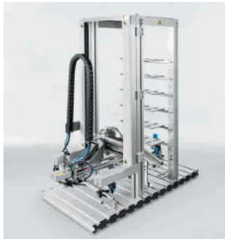
Fig. II.9: Station stockage et déstockage
