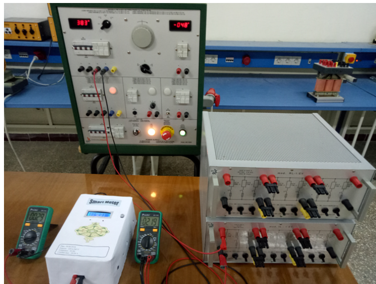
FIGURE III.11 – Alimentation de la charge inductive.
