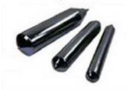
Figure II-5 : Lingots de silicium monocristallin [12]
