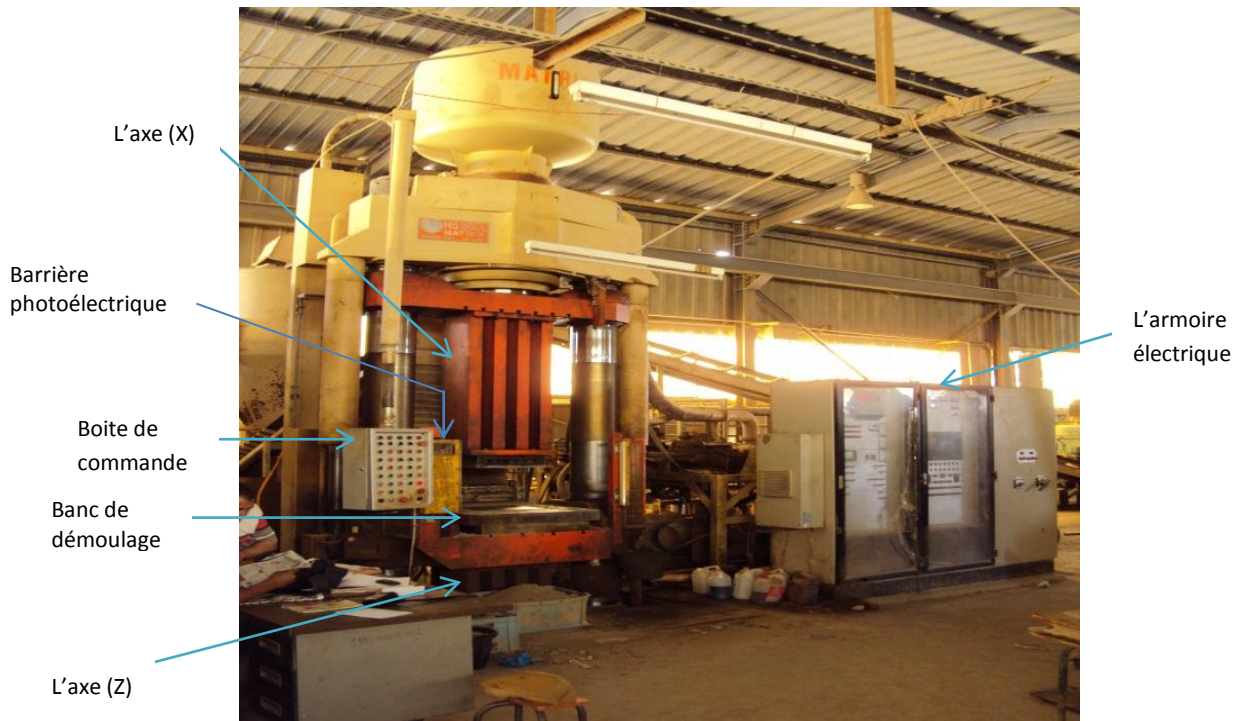
Figure 2.1. La presse MATRIX HS 550L
