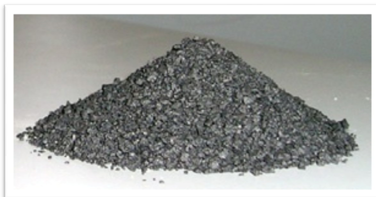
Figure 3.10 :Backfill de coke (12).
