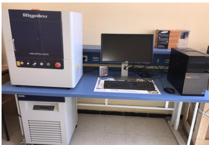
Figure II.5. Appareil DRX ‘ Rigaku MiniFlex 600’
