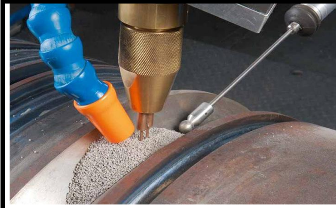
Figure 05 Arc submergé (SAW)
