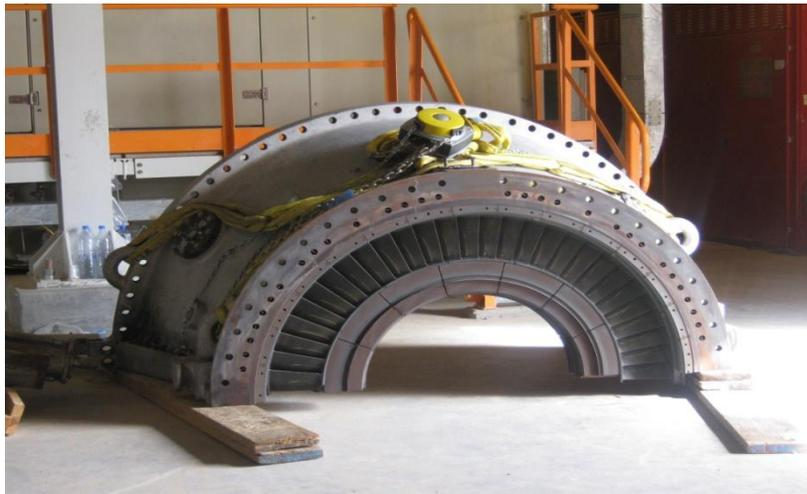
Fig.22 Stator de la turbine
