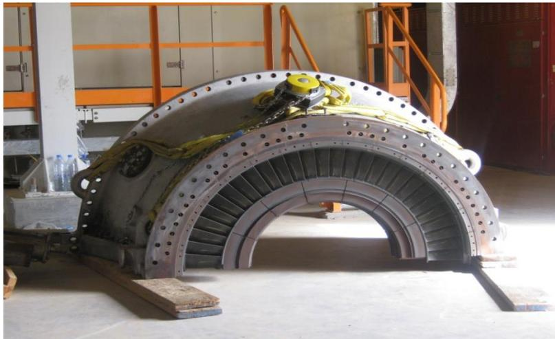
Fig.22 Stator de la turbine
