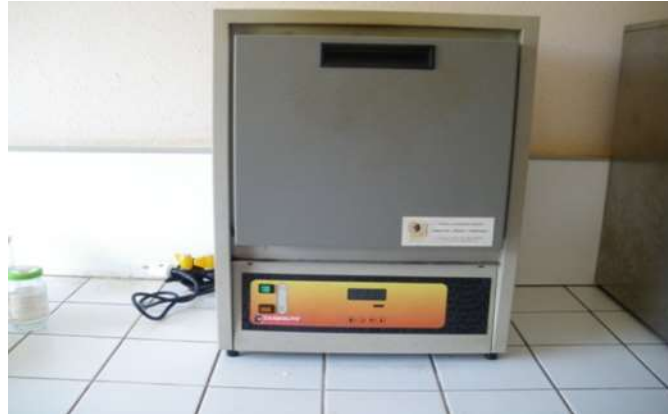
Figure III-6: Four à moufle (Photo originale)
