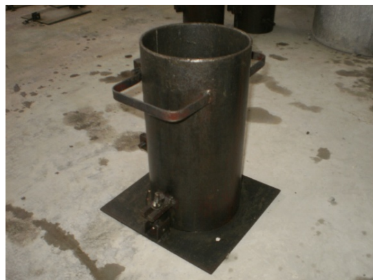
Figure 2. 2 Moule cylindrique 16x32 (cm)
