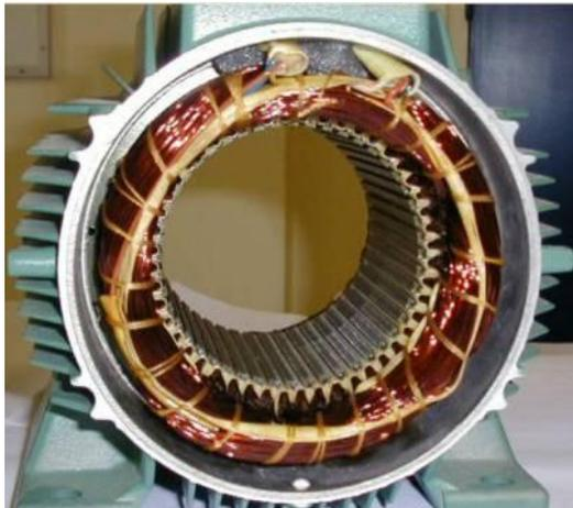
Figure I.2.a: Stator [11]
