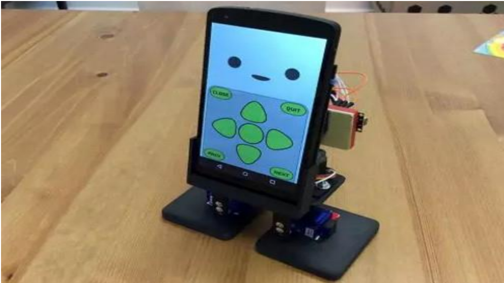
Figure 1.2 : "MobBob" - the intelligent Android Mobile Phone Robot
