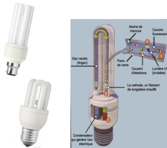
FIGURE II.14 – Lampe fluorescente compacte
