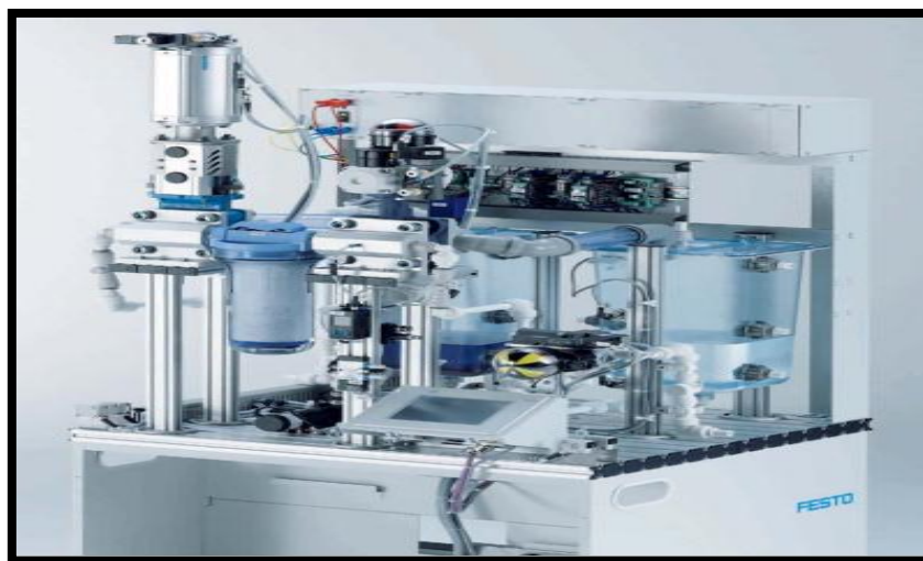
Figure 3.2 : station de filtration
