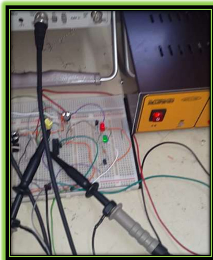
Figure 5 :le clignotement de la led D1
