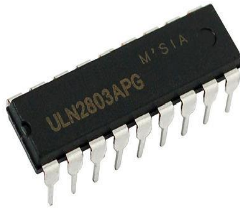
Figure 20: le circuit ULN2803[4]
