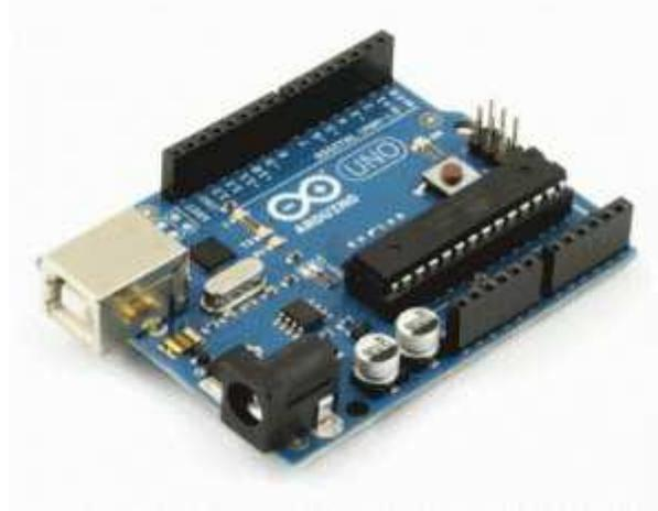
A blue Arduino Uno R3 microcontroller board with various components like a USB Type-B port, a DC power jack, and several integrated circuits. |
