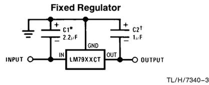
\*Required if regulator is separated from filter capacitor by more than 3". For value given, capacitor must be solid tantalum. 25  $\mu F$  aluminum electrolytic may be substituted.
