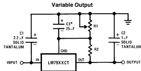
\*Improves transient response and ripple rejection. Do not increase beyond 50  $\mu\text{F}$ .
