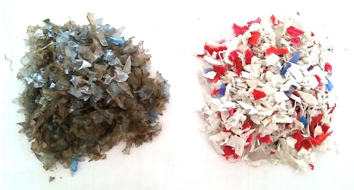
Figure 3.16 MATIERE OBTENUE APRES BROYAGE
