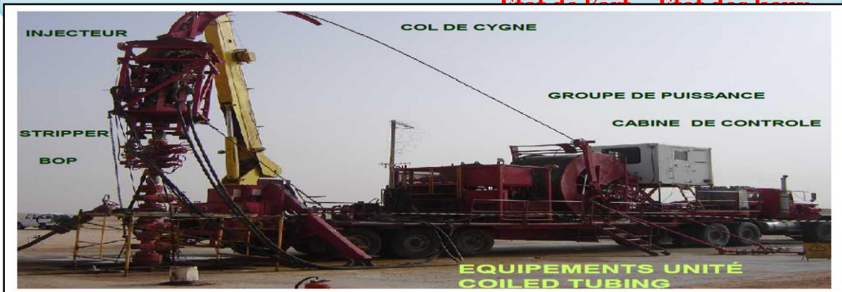
Figure 12: Equipment d'une unité de COILED-TUBING
