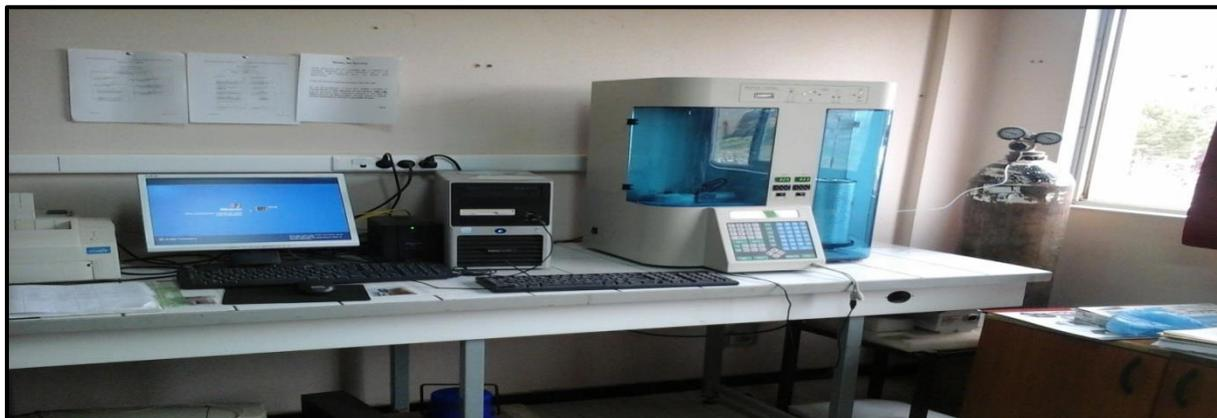
**Figure4:** Appareil micromeritics NOVA 1000<sup>e</sup>.
