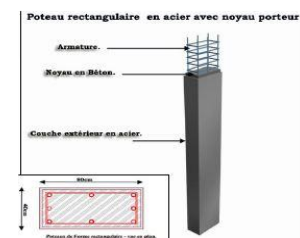
Figure: poteaux rectangulaire
