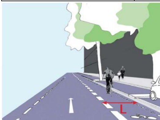
Figure 159: dimensions bande cyclable. Source: https://www.grandlyon.com
