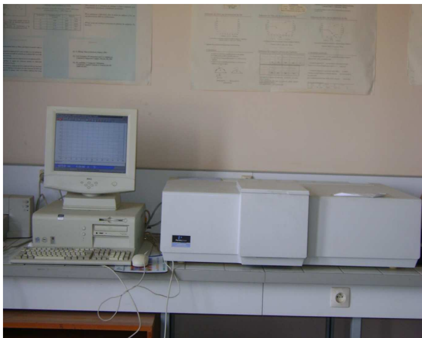
Figure 6: Appareil de l'Ultraviolet-visible, Lambda 800
